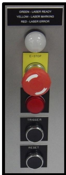
Front panel lights and buttons for intuitive and safe operation.
